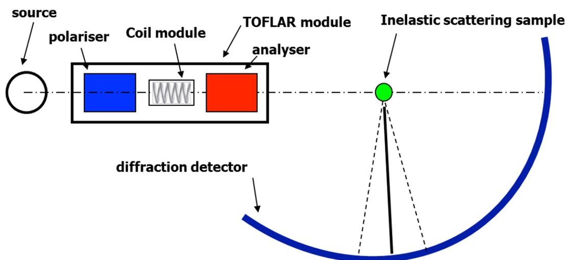
*Fig. 6: Schematic drawing (not in scale) of a TOFLAR module introduced at the incoming beam of a powder diffractometer. The module consists of a precession field between a polariser creates an intensity modulation as a function of wavelength and magnetic field. Due to inelastic scattering the amplitude of this modulation will decrease.*
